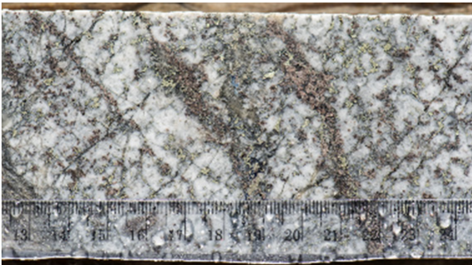
Quartz vein in the Main Zone with cassiterite (tin oxide, pale purple-brown colour) and sphalerite (indium bearing zinc sulphide, dark to black colour)
