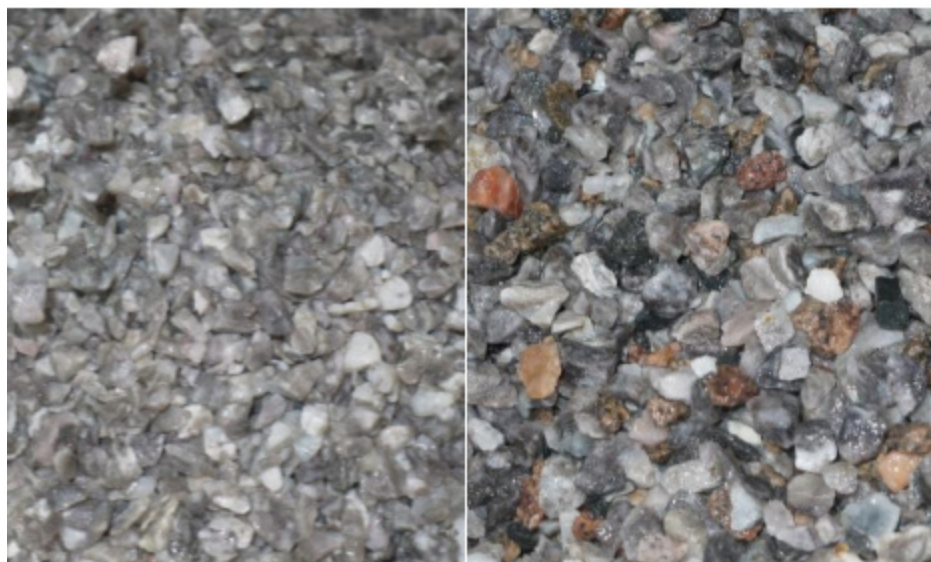
Crushed ore from the Separation Rapids deposit after it has been optically sorted. The “cleaned” ore is shown on the left. The discarded waste material shown on the right is noticeably darker and more brightly coloured.
